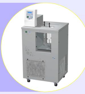
Top lid stainless steel Integrated cooling High precision better than ± 0.02°C Large windows, no condensation Easy to operate RS232 communication
